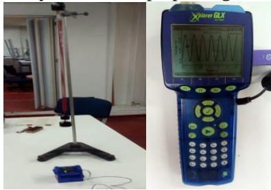
Fig. 5 Experimental setup for strategies 3 and 4 in the laboratory; materials and equipment used: universal support, PASPORT motion sensor (placed below the mass), and Xplorer GLX - PS-2002 reader
